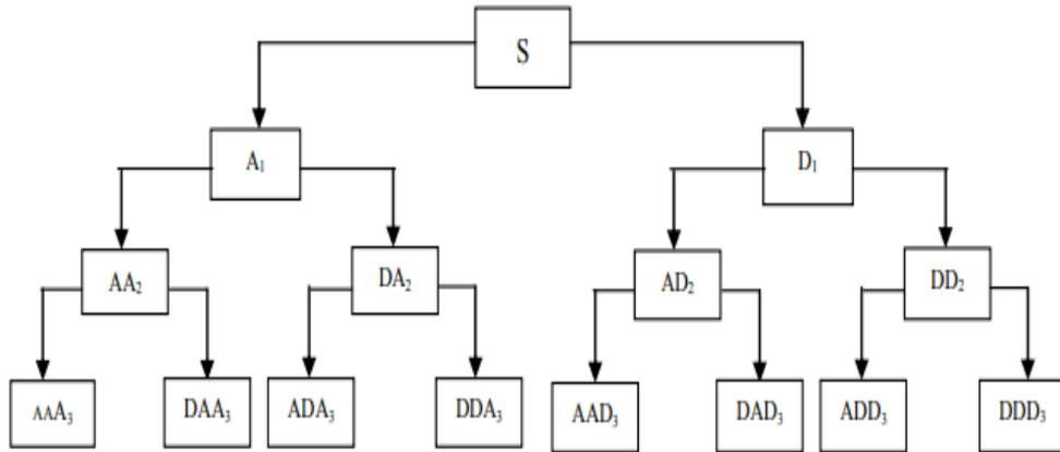
**Fig. 3.** Wavelet Packet Decomposition Process
