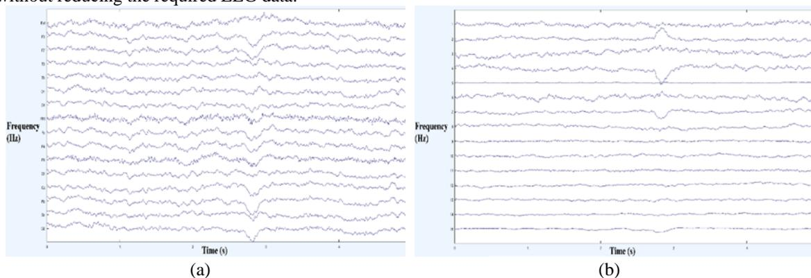
**Fig. 4.** Preprocessing Data (a) before using ICA (b) after using ICA
